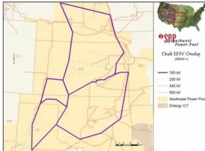
*Long-term vision of a 765-kV transmission overlay that would provide the ability to develop these resources and move power freely across the entire SPP footprint.*
